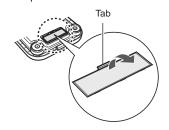
2. Install the batteries in correct polarity as marked inside the battery compartment.
